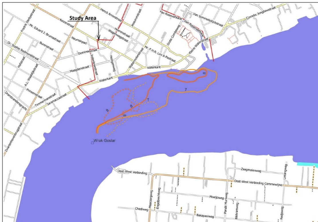
Figure 23. Comparison of the 7m and 8m depth contour lines of 2022 with the 1993 ones
