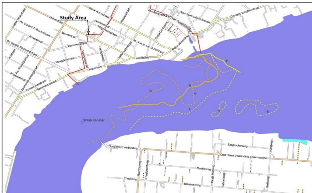
Figure 5-32: Comparison of the 5 m and 6 m depth contour lines of 2022 with the ones of 1993.
