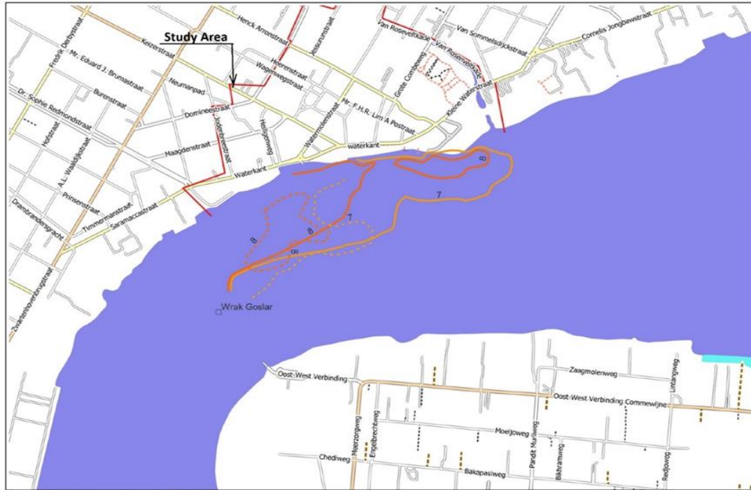
Figure 5-31: Comparison of the 7 m and 8 m depth contour lines of 2022 and 1993.
