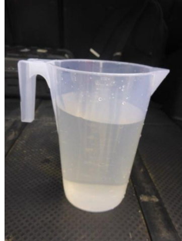
Location WQ9: Color of the collected water is very light brown. Clarity of the water is almost clear.
