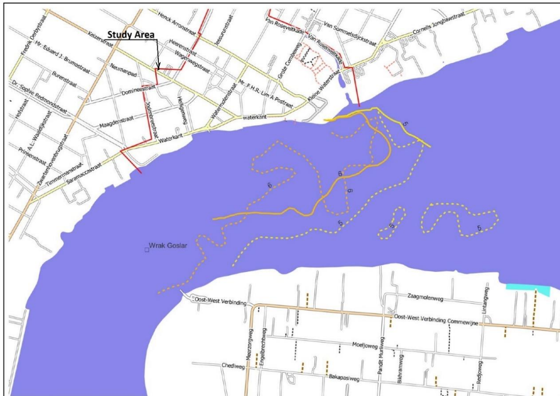
Figure 24. Comparison of the 5m and 6m depth contour lines of 2022 with the 1993 ones
