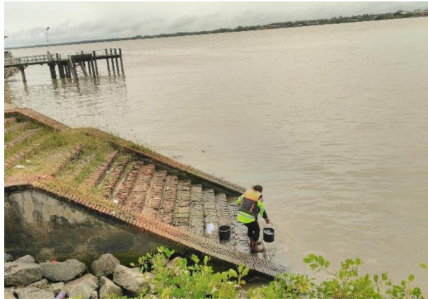
Location WQ3: Collecting water in the Suriname River at the Marine trap during the rising from low to high tide.
